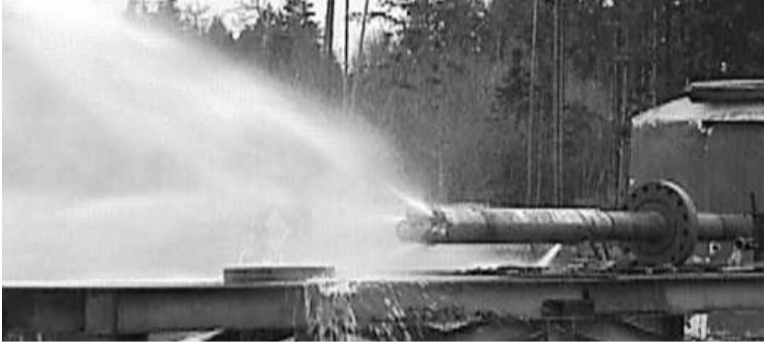
Figure 2. Cycling valve tests of full-scale suction pulse tool equipped with 222 mm bit.
