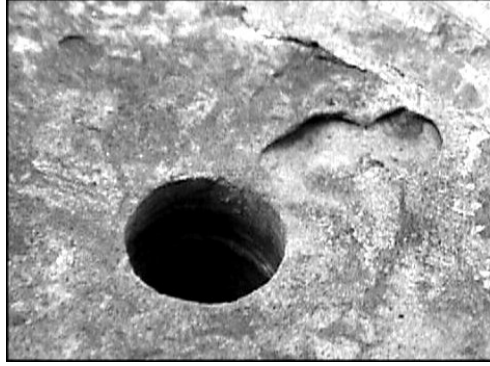
Figure 8. Surface pit in Mancos Shale sample after suction pulse drilling experiment. Pit is above and to the right of the 8.7 mm diameter borehole.
