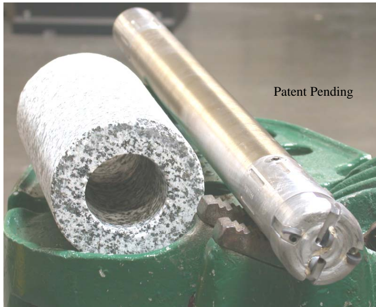
Figure 3. Tempress Jet TurboDrill™ with jet-assisted PDC bit.
