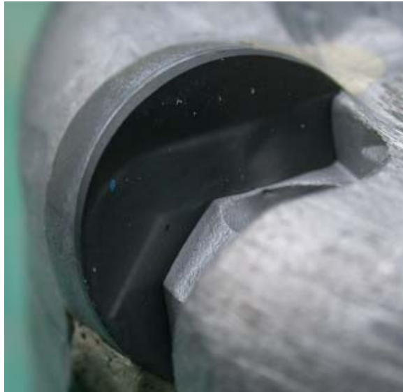
Figure 14. Wear flat on gage PDC cutter.
