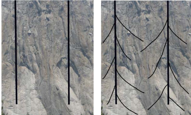
Figure 1. EGS injector/producer pair (left) with multilateral network (right)
