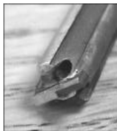
Figure 12. Microbit with 20 degree backrake carbide cutter.
