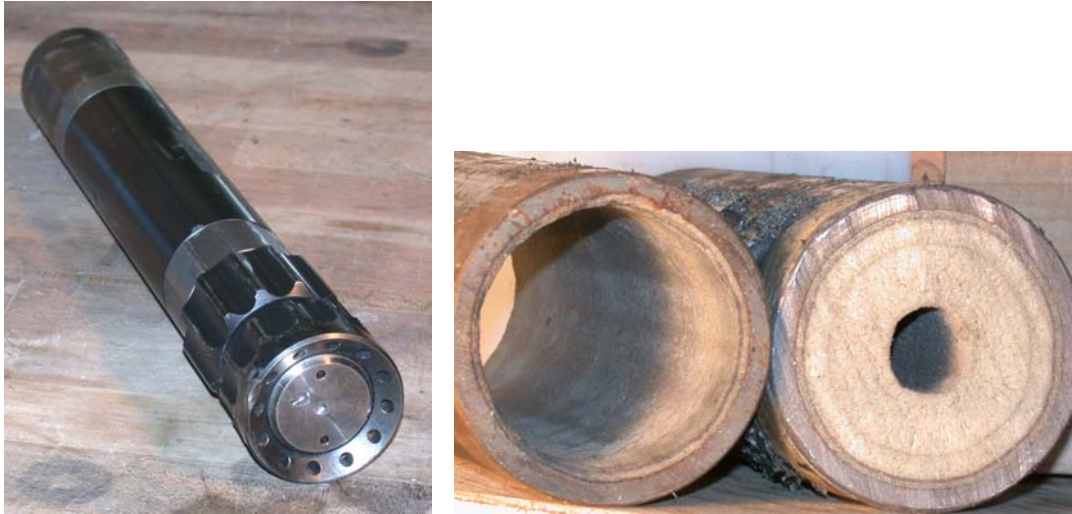
Figure 9. High pressure jet drill and 2-1/4" hole milled in hard carbonate scale at 35 MPa.
